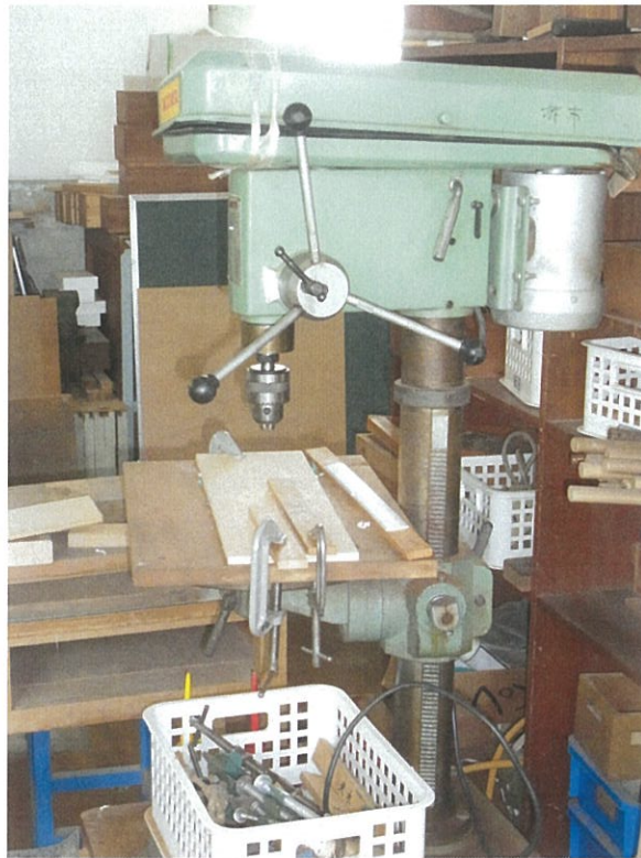
FIGURE 16. A device that bores holes in rubber closures.
