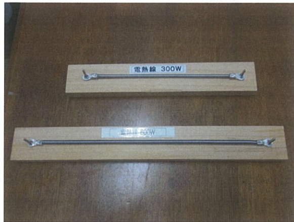
FIGURE 11. A heating wire that wouldn't stretch because of a thin strip of bamboo.
